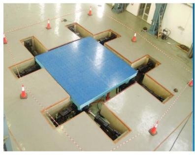
Shaking table, is a device used in seismic testing to simulate earthquake conditions and evaluate the response of structures or materials to these dynamic forces. It allows researchers to study how buildings, components, or even soil behave under earthquake-like vibrations.
