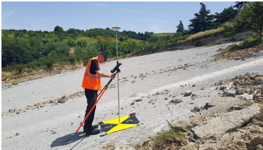
GNSS survey on translational slide at Fontanelice (BO)
