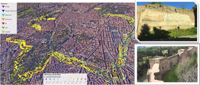
Rome Walls deformation satellite monitoring © Spizzichino
